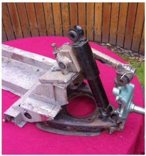
The part of the turret which has been cut off is replaced with a plate welded in place to create a strong box structure. The new turret (A) is designed to sit on top of the existing turret. It bolts directly to where the original lever arm was situated. It also locates the two piece wishbone (B) and supports the top of the coilover. (C) A bracket is located at the base of the upright in the existing bottom wishbone to take the end of the coilover. (D)
