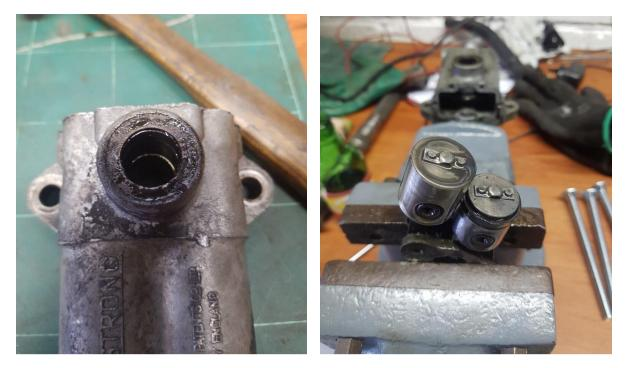
With the shaft removed the remains of the felt seal could be pried out and the crank / piston assembly removed. The pistons are handed, one with a rubber seal, so again the orientation was noted. The bores and piston pins were checked and found to be free of wear which was good news. To restore the damper body I mounted it onto the faceplate of my Myford lathe and clocked in on the seal bore. The main bores were too badly worn to be sure of the original position.
