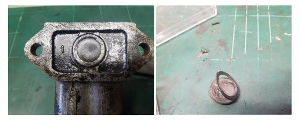
The back of the shaft could now be accessed. The damper was set up carefully on the press and the shaft pressed out. Care was taken to support the casting to prevent it distorting. I made sure to note the orientation of lever arm relative to the crank inside the body.
