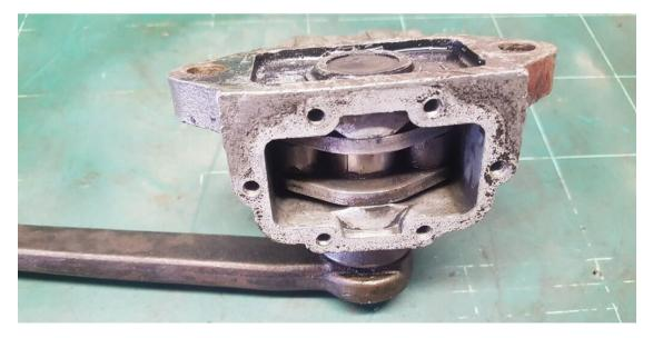
The shaft needed to be pressed out. To access it the plug needed to be removed. This was a press fit with the body swaged over behind it so required some Dremel and pry bar action
