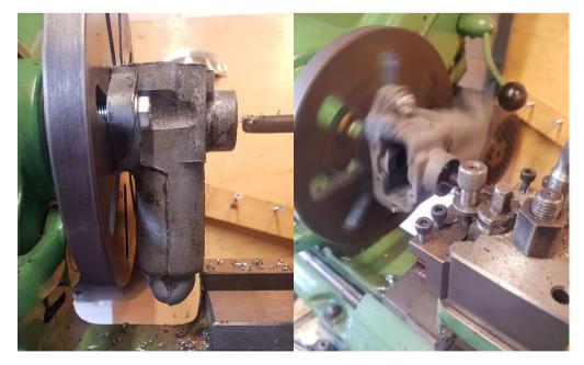
A tight fit. I bored the housing to accept Acetal bushes. Phosphor bronze or brass would probably have worked just as well. I also rebored the front to accept an SKF shaft seal (25X40X7 CRW1 R) to replace the felt.
